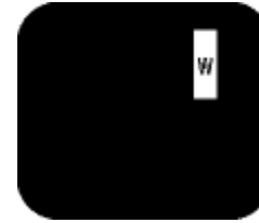
Three adjacent lit subpixels (one white pixel)
